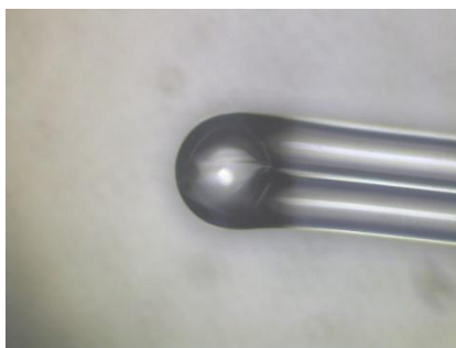
Figure 1. Optical microscopy of dual fiber probe.
